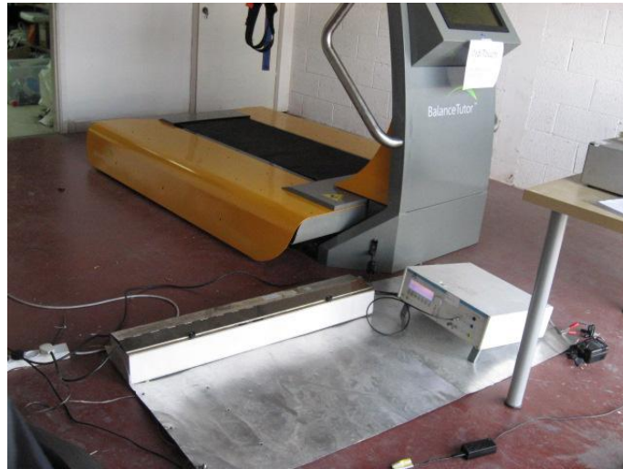
Figure 17. Immunity to Electrical Fast Transient / Burst Test
