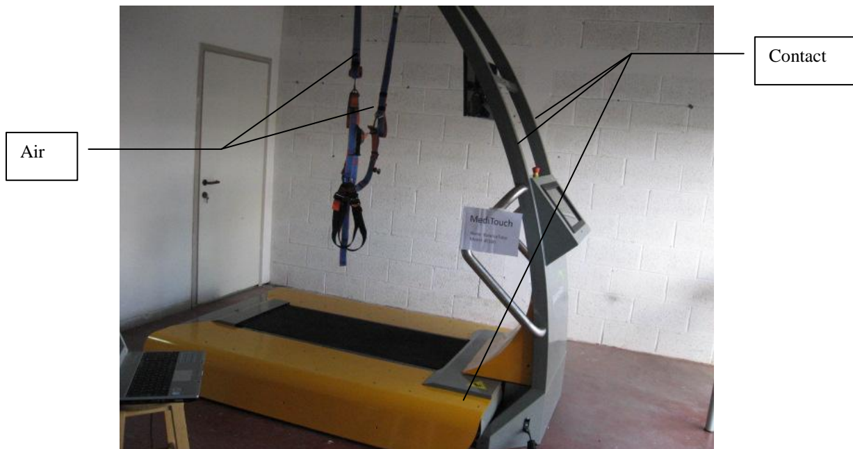
Figure 10. ESD Test Points
