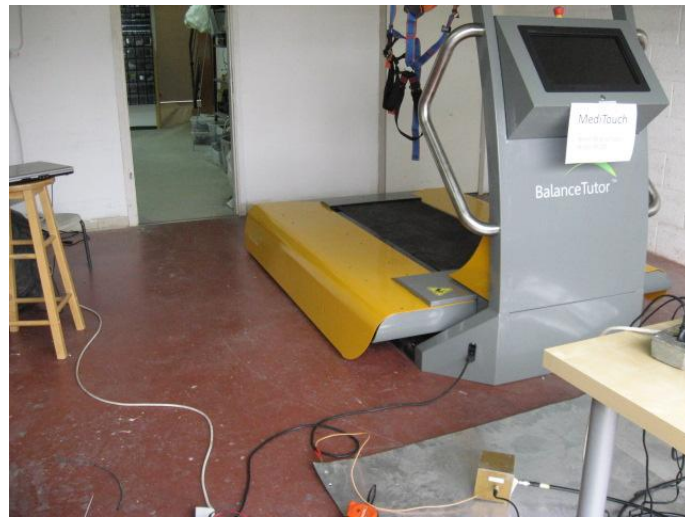
Figure 13. Conducted Emission From AC Mains Test
