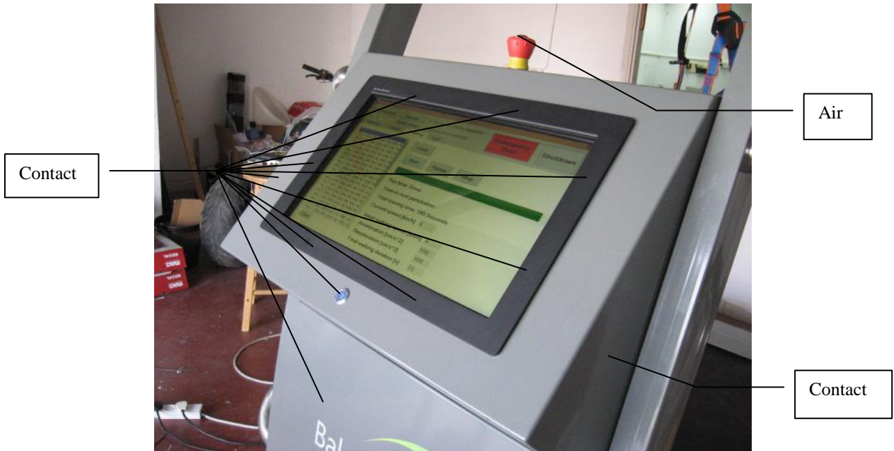
Figure 8. ESD Test Points
